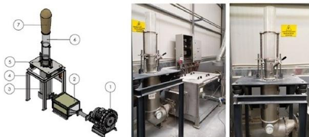
Fig. 1. Fluid bed dryer (1: Fan, 2: Resistance heater, 3: Hot air channel, 4: Dryer stand, 5: Product chamber, 6: Drying chamber, 7: Filter).
