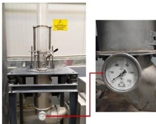
Fig. 3. Sub-sieve pressure measurement manometer.
