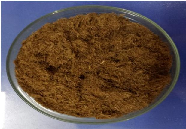
Figure S2. Rice straw sample after physiochemical pretreatment with 2% H<sub>2</sub>SO<sub>4</sub> at 121oC for 90 mins.
