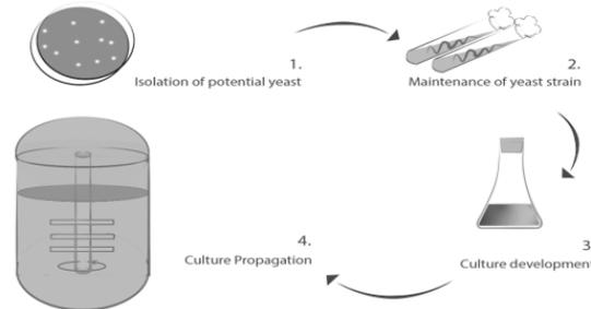
Figure S4. Sequential steps for inoculum preparation for fermentation.
