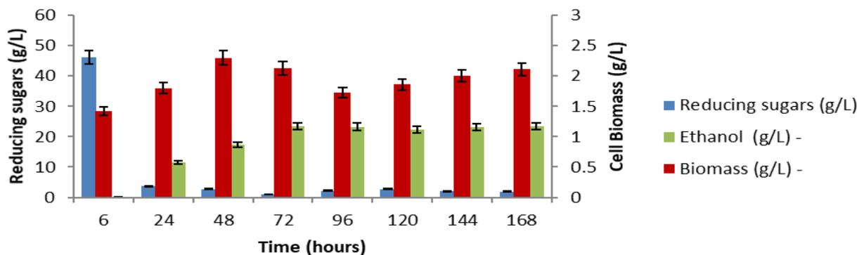
Fig. 10. Semi continuous Fermentation for bioethanol production in fermentation medium using *S. cerevisiae* ML-6.
