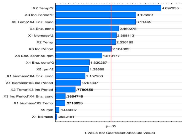
**Fig. 3. Pareto chart showing t-value coefficients for total sugars at 0.05 sigma restriction generated by Statistica v.10.0.1.**
