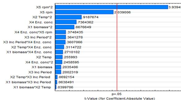
**Fig. 1. Pareto chart showing t-value coefficients for reducing sugars at 0.05 sigma restriction generated by Statistica v.10.0.1.**
