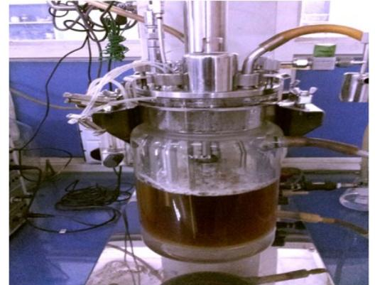
Figure S6. Batch fermentation using *Saccharomyces cerevisiae* ML-6 in fermentation medium.
