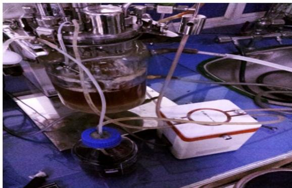
Figure S7. Semi continuous process using *Saccharomyces cerevisiae* ML-6 in fermentation medium.
