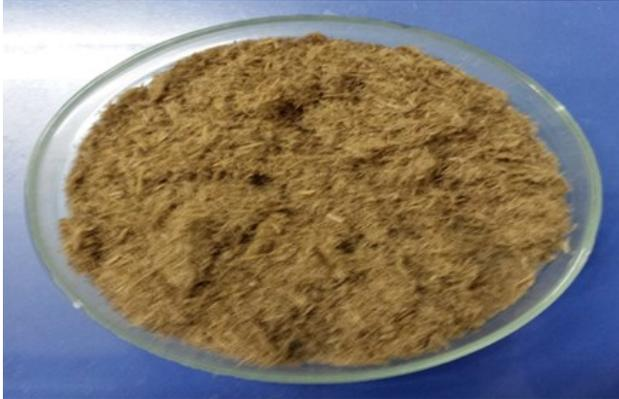
Figure S1. Physically treated (crushed) sample of 2 mm mesh size rice straw.
