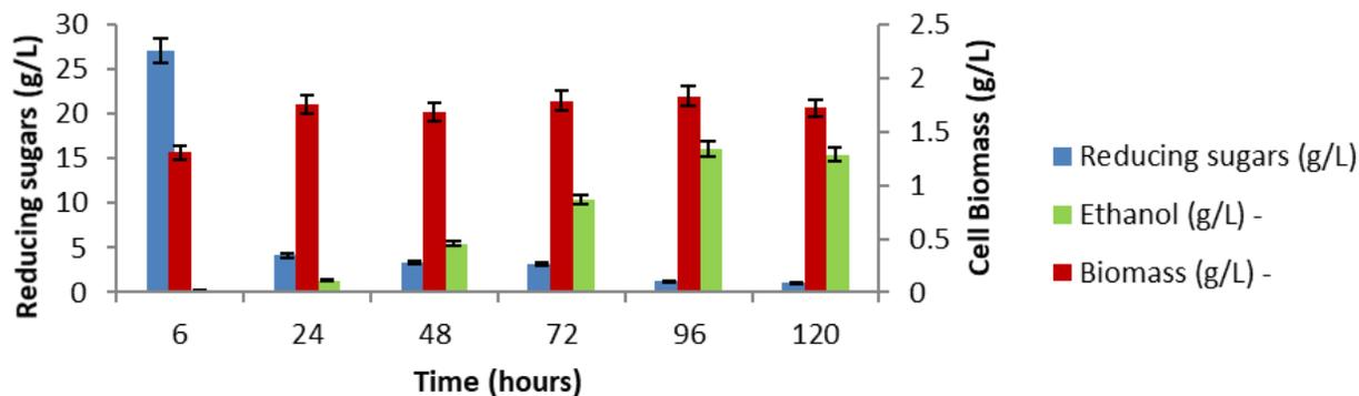
Fig. 8. Batch Fermentation for bioethanol production from Saccharified Rice Straw Hydrolyzate using *Saccharomyces cerevisiae* ML-6.
