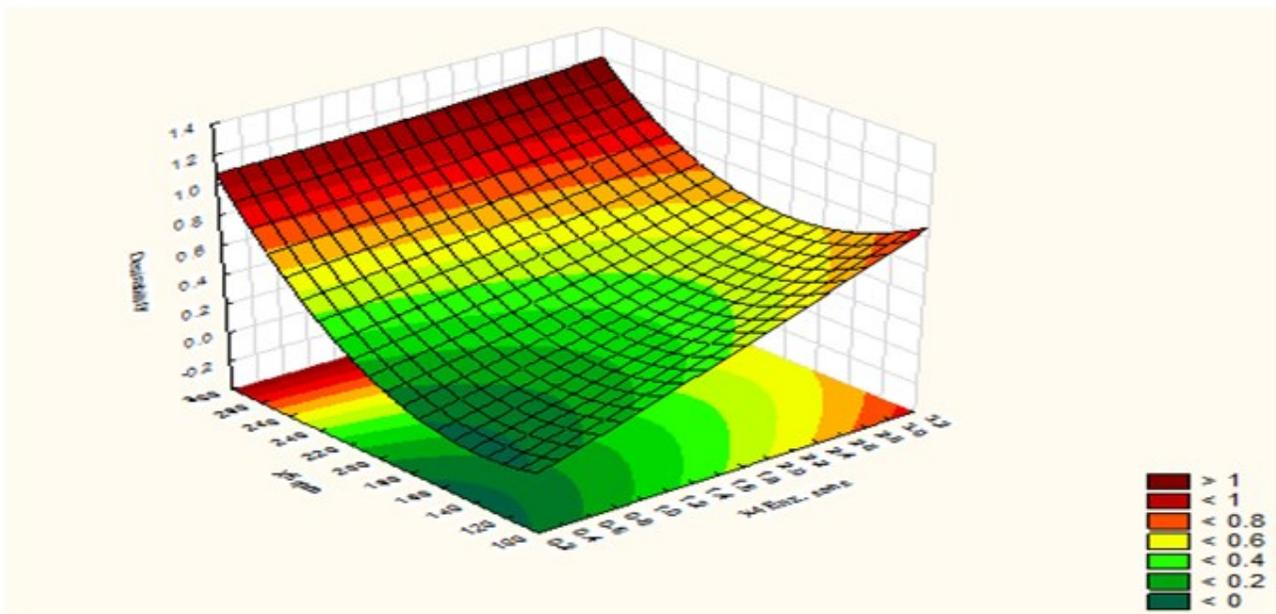
**Fig. 2. Response surface plot showing effect of interaction between Enzyme concentration (X4) and Agitation speed (X5) on Reducing sugar yield generated by Statistica v.10.0.1.**
