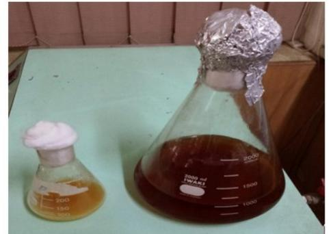
Figure S5. Inoculum of *Saccharomyces cerevisiae* ML-6 (left) and fermentation medium (right).
