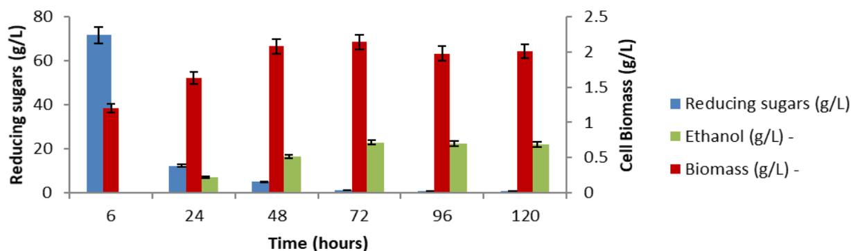
Fig. 9. Batch Fermentation for bioethanol production from Saccharified Rice Straw Hydrolyzate supplemented with Glucose using *Saccharomyces cerevisiae* ML-6.
