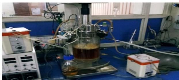
Figure S8. Continuous process using *Saccharomyces cerevisiae* ML-6.
