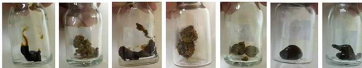
Fig. 1. (Left to right) Crude extract for stability testing and triturated kollidon, starch, PVP, microcrystalline cellulose (MCC), talc, and lactose for compatibility testing.
