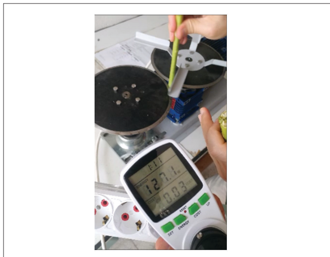
Fig. 7. Cutting energy measurement with electricity consumption measuring device.
