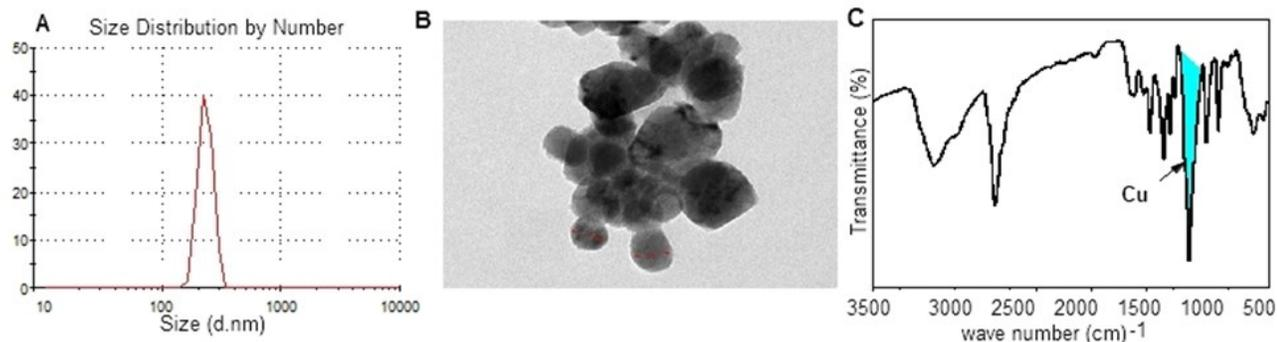
**Fig. 1. A:** Dynamic light scattering (DLS) of chemically-produced copper nanoparticles (CuNPs), **B:** Transmission electron micrographs (TEM), **C:** Fourier transform infrared (FTIR) spectroscopy of synthesized CuNPs.
