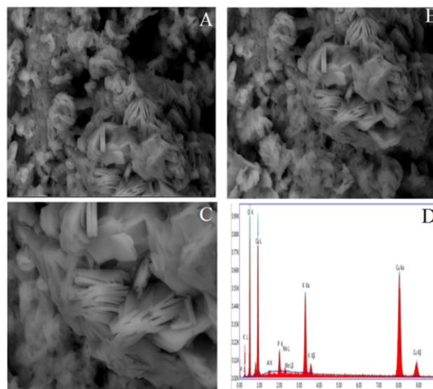
Fig. 2. Scanning electron microscopy (SEM) images A, B: mag 8000x, C: 16000x, D: energy dispersive X-ray spectroscopy (EDX) spectra of synthesized copper nanoparticles (CuNPs).
