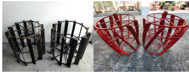
Fig. 1. Conventional (left) and modified (right) cage wheels.
