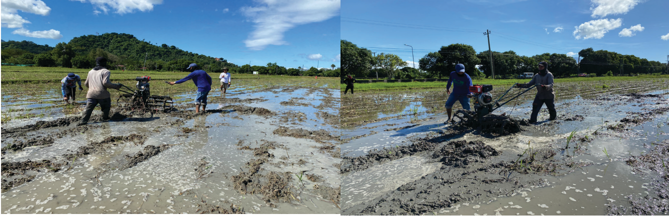
Fig. 5. Actual field test of the conventional (left) and modified (right) cage wheels.
