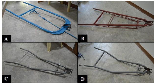
Fig. 1. Handlebar designs used in the study: Original handlebar design (A), B-K Design 1 (B), B-K Design 2 (C), and the proposed design (D).
